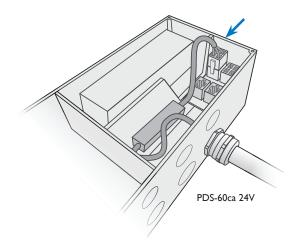
5. Secure the power / data supply cover. If installing in a wet or damp location, seal the power / data supply with electronics-grade RTV silicone sealant.
