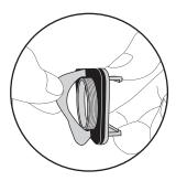
3. Insert the lens or glare shield holder through an opening in the substrate, and temporarily affix the lens holder by pressing the adhesive surface to the back of the substrate. Make sure that the holder is oriented in the direction of the iColor Flex LMX gen2 strand.
