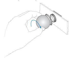
• Align the tabs on the glare shield with the slots in the glare shield holder, and snap the glare shield onto the glare shield holder.
