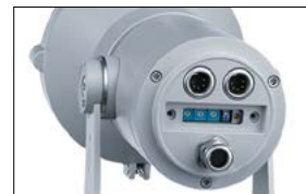
Easy addressing: addressing in the case of PYLAS L RGB and PYLAS XL RGB is performed easily via three rotary switches that are accessed by unscrewing a cover.
