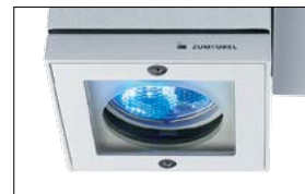
Flush-fitted glass diffusers with no raised luminaire frame prevent dirt accumulation and the reduced light that this causes. The luminaire is almost self-cleaning.
